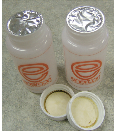
Excessive wrinkling, signs of burning or discoloration on either the liner or in the cap indicates that either the output is set too high or the line speed is too slow.
