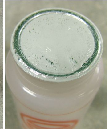
Excessive wrinkling, signs of burning or discoloration on either the liner or in the cap indicates that either the output is set too high or the line speed is too slow.
