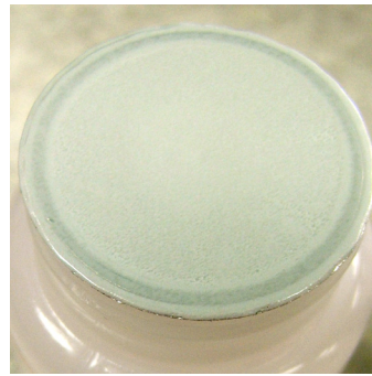
A good seal exhibits adhesion around the circumference of the container, no discoloration and minimal wrinkling.
